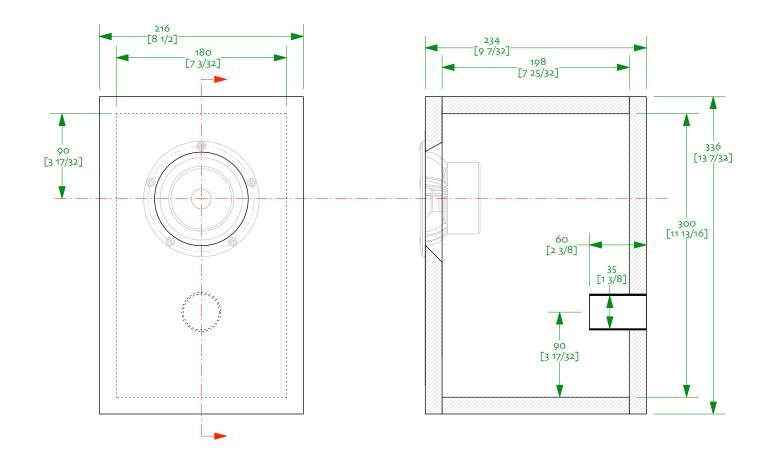
o/ Compact vented box standmount for Mark Audio Alpair 7MS 4in negative-camber wideband drive unit – 10.5 litres
